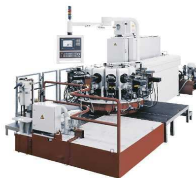
Machines Transfert - Transfert Maschinen Transfer Machines
